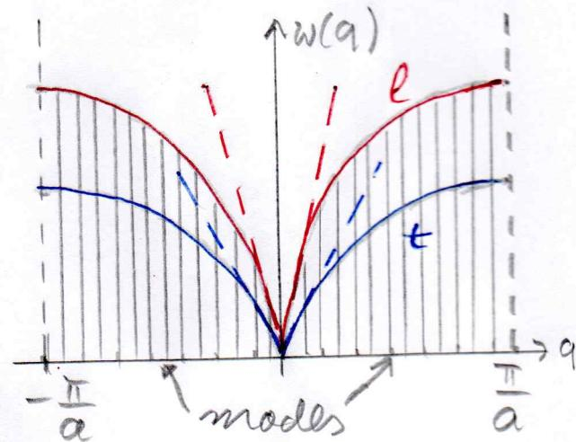
the latter defining the sound velocity in the continuum limit. One distinguishes between longitudinal lattice vibrations (—) with the dispersion  $w_e = w_e(\vec{q})$  and transversal lattice vibrations (—) with the dispersion  $w_t = w_t(\vec{q})$ , which is doubly degenerate. In general we have
