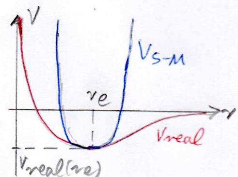
Expanding the potential  $V_{\text{real}}$  around the equilibrium  $r_e$  up to second order, one obtains the harmonic approximation  $V_{\text{s-m}}$  (—):
