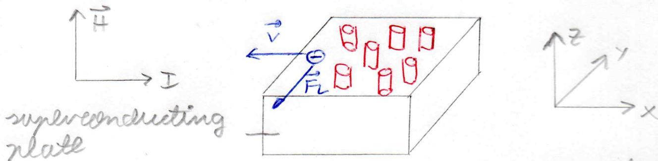
The flux lines penetrate the plate from the bottom to the top. Here it is essential that the external magnetic field goes basically unaffected through the core of the flux lines.
