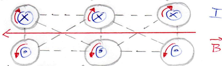
For the construction of a superconducting coil one has, therefore, to take into account the fact that the critical current at a winding is smaller than the corresponding critical current at a single winding:
